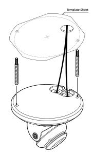
3 Pull wires through and make all necessary connections. See the section '6. Cabling' for details.
