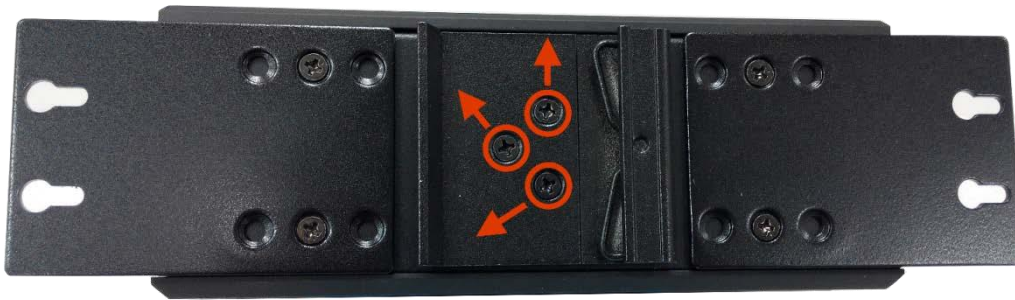
Figure 3.4: Remove DIN-Rail Bracket from the Switch
