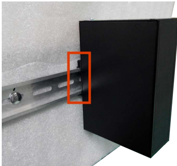
Figure 3.3: Stable the Switch on DIN-Rail
