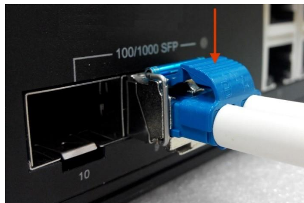
Figure 2.4: Remove LC Connector
