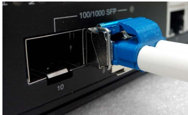
Figure 2.9: LC Connector to the Transceiver
