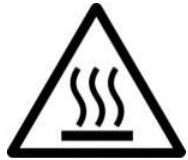
Figure 1.2: Hot Surface Warning Label
