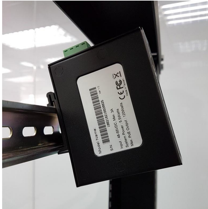
Figure 3.2: Insert the Injector on the DIN-Rail
