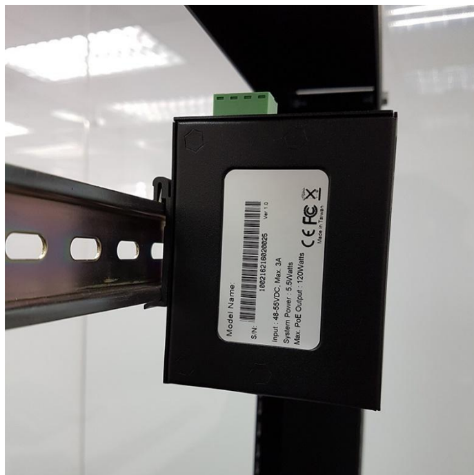
Figure 3.3: Stable the Injector on DIN-Rail
